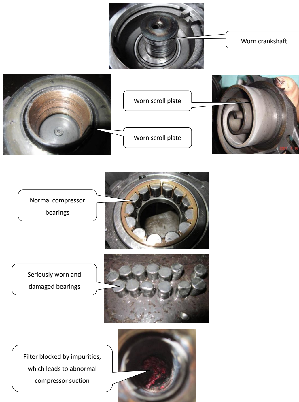
Figure 6-2.11: Effects of spoiled compressor oil
