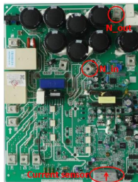
Figure 6-2.2: DC detection wire connection method
