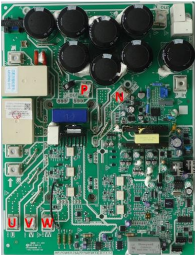
Figure 6-2.7: Inverter module terminals
