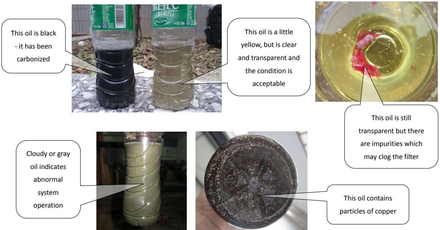
Figure 6-2.10: Inspecting compressor oil
