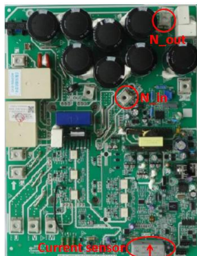
Figure 6-2.5: DC detection wire connection method
