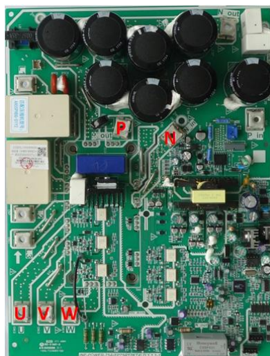
Figure 6-2.6: Inverter module terminals
