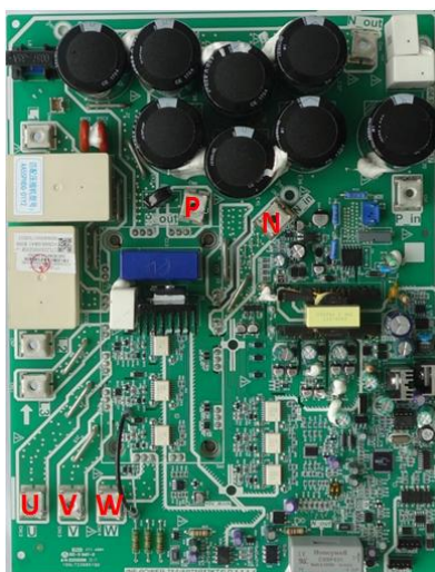
Figure 6-2.1: Inverter module terminals
