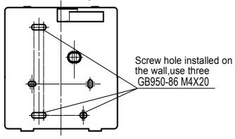
3) Use two M4X25 GB823-88screws to install the back cover on the 86 electrician box, and use one GB950-86 M4X20 screw for fixing the wall.
