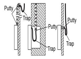
3) Avoid water enters into the wired controller, use trap and putty to seal the connectors of wires during wiring installation.
