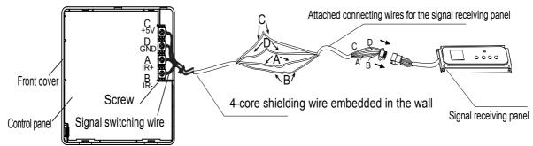
2) If embedded 4-core shielding wire cannot go through the wired controller, it can use signal switching for connection and make sure the wires are reliable and firm. The tightening torque range of the screw is0.8~1.2N .m (8~12 kgf . cm).
