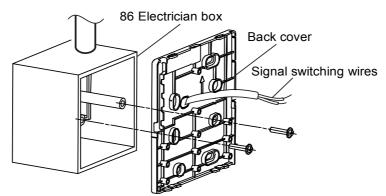
**Notes:** 1.Use cross head screws to fix the wired controller bottom cover in the electric control box through the screw bar. Make sure the wired controller bottom cover is on the same level after installation, and then install the wired controller back to the bottom cover.
