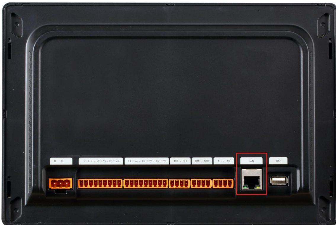
(Highlighted is the LAN port of CCM-270A/WS)
